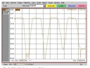
Fig 2. S21 'Odd' channels 'ON'
